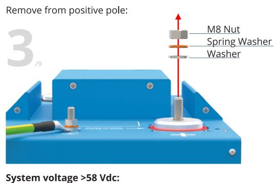
Replace battery pole + fuse with the non-fused battery pole.
